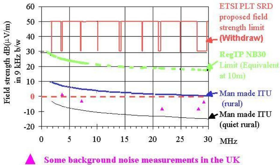
This illustration shows the relative level of the proposed NB30 limit. At this level only the strongest HF radio signals can be heard above the PLC systems.
