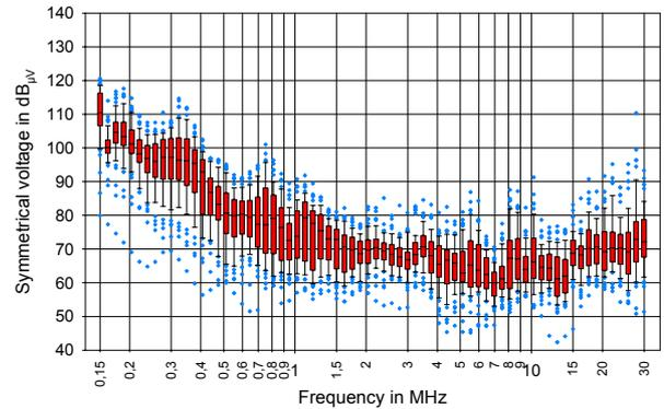
**Figure 7** Symmetrical Voltage that leads to magnetic fields according to the German regulation NB 30
