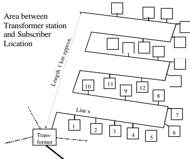
Fig 1: Structure of the low-voltage power supply network in dwelling areas
