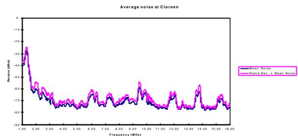
Fig 2: Mean values of disturbance from 20-ms sweeps at 9 locations of a British town [4] (100 kHz measurement bandwidth and peak detection). For 10 kHz bandwidth the level will therefore be 20 to 30 dB $\mu$ V.
