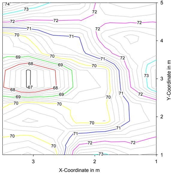
**Figure 5** Local distribution of the magnetic field when a symmetrical voltage of 105 dB<sub>µV</sub> is coupled into the power line at (0,0), z = 1 m
