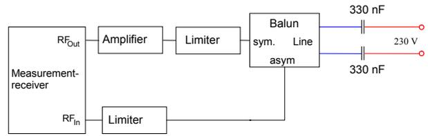
**Figure 1** TCL measurement setup
