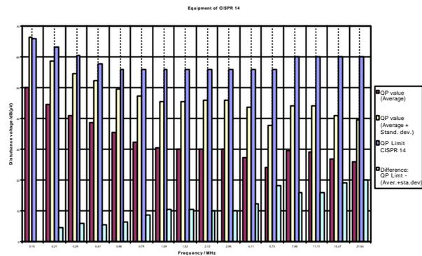
Fig. 5: Mean values of RFI QP voltage and mean + standard deviation of 35 different types (140 units) of household equipment and portable tools (CISPR 14 equipment). The frequency range was divided in 16 logarithmically equal subranges. In each subrange the maximum voltage relative to the limit was used for the statistical evaluation. The QP emission limit is added for comparison. (Data received from RegTP).
