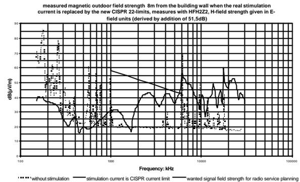
Fig 3: Values of field strength measured with a loop antenna at 8 m distance from a three-storey building. Dotted line: ambient emission; thin continuous line: field strength generated by injection of the common-mode current equivalent to the CISPR22/EN55022 emission limit into the telecommunication network of the building; bold line: minimum useable field strength for radio planning. HFH2-Z2: R&S active loop antenna 9 k to 30 MHz. (Measured data received from the RegTP)
