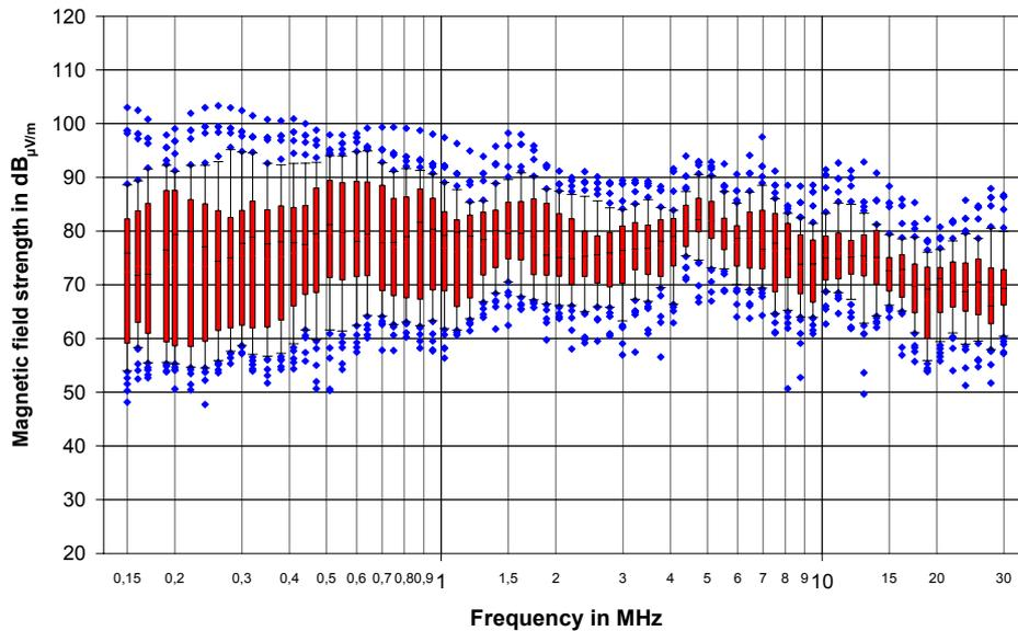
**Figure 2** Measured field strength  $H$  in a distance up to 3 m of the coupling point when a symmetrical signal of  $105 \text{ dB}_{\mu V}$  was coupled into the power-line
