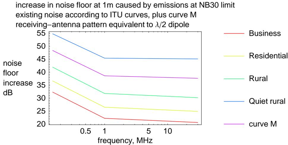
The *smallest* noise-floor increase arises where existing the indoor noise corresponds to ITU-R “Business”, and is then 20 to 33 dB. Other regions suffer greater noise-floor increases, up to 55 dB! In comparison, the plot presented in § 3.4. shows that the new proposal causes *at most* an increase of about 18 dB at 1 m.
