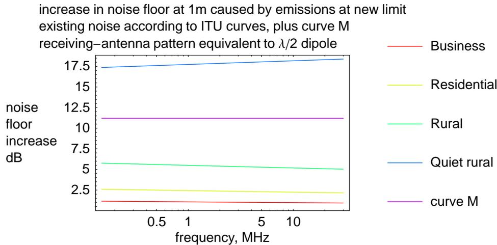
The compromise inherent in the new proposal is now clear. Those locations where pre-existing noise levels indoors remain low will be significantly affected. Note that this compromise will primarily be made by broadcasting, since it is the radio service in this frequency range for which indoor reception is most used and expected.
