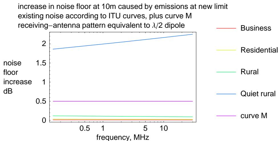
The increase is 0.5 dB exactly for curve M (just as we designed it). Where the existing noise floor is lower (e.g. ITU-R “Quiet rural”) the increase is greater, while for areas where the existing noise level is worse than curve M the increase is negligible. We may conclude that outdoor-antenna reception is, as intended, well protected by the new limit proposal.
