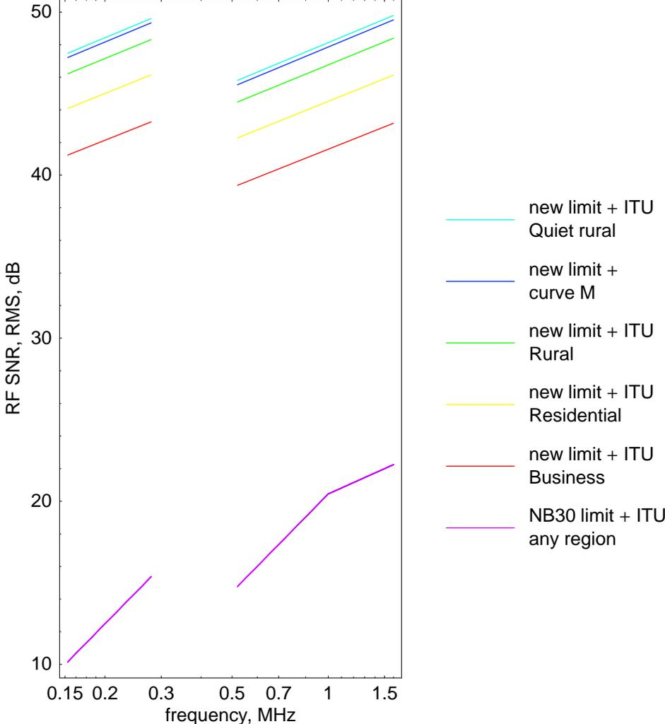
The 40 dB RF SNR target is essentially met under the new limit, for all ITU noise regions, whereas the NB30 limit falls short by up to 30 dB.
