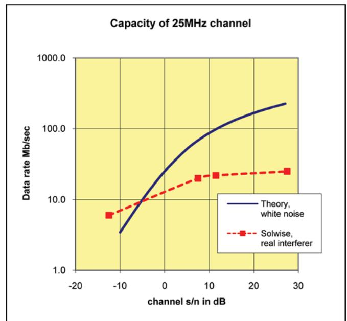
Figure 2. The capacity of a communication channel in the presence of interference.
