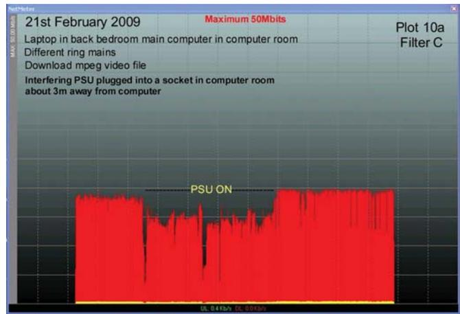
Figure 4. Turning on a local interferer reduced the throughput from 18Mb/sec to 13Mb/sec.
