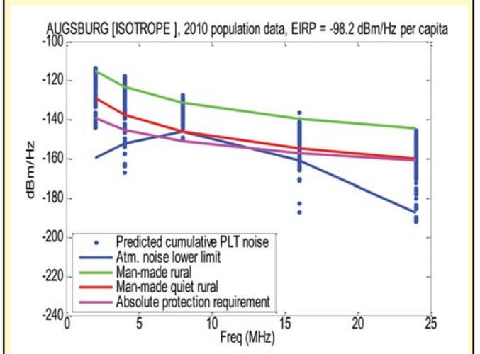
**Figure 6 Predicted cumulative PLT noise parameters for example with receiver in Augsburg, compared to established background noise levels.**
