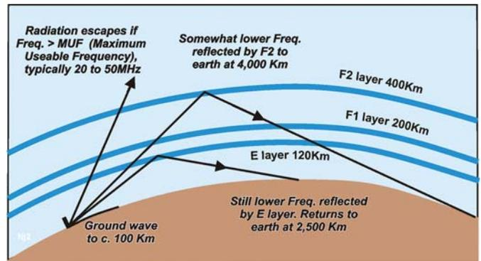
**Figure 3** The geometry of radio wave propagation (not to scale)
