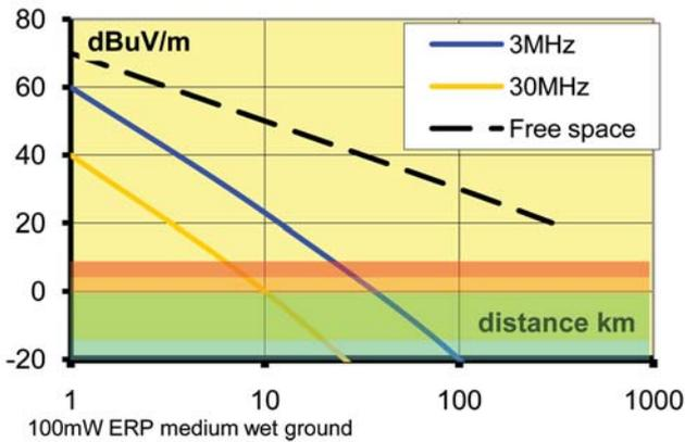
**Figure 1** The signal strength of a 100mW source compared with the noise background. The red background corresponds to a “business” environment, the orange to “residential”, the green to “Rural” and the blue to “quiet rural” at 10MHz
