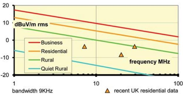
**Figure 2** Man-made noise levels in various environments. This data is derived from ITU R372-9 figures for median external noise figure, assuming use of a half-wave dipole and 9kHz bandwidth. Note that above 10MHz galactic noise is some 5dB above the man-made “Quiet rural” level shown here.
