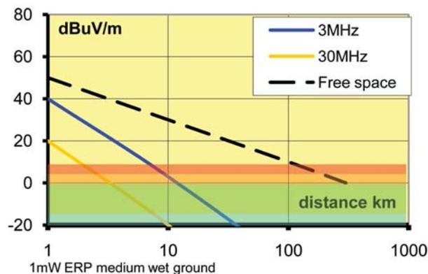
**Figure 5** Field strength resulting from a 1mW transmitter. As in Fig 1 the red background corresponds to a “business” environment, the orange to “residential”, the green to “Rural” and the blue to “quiet rural”
