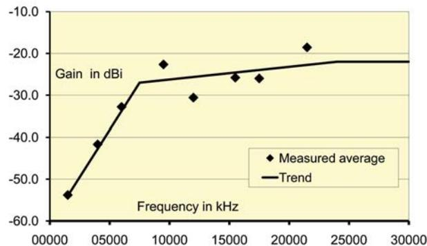
**Figure 4 Average sky wave antenna “gain” for indoor sockets.**
