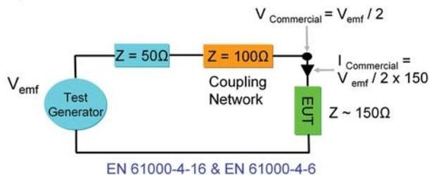
Figure 8 – Coupling Device Correction
