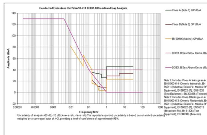
Figure 4 – Example Broadband Emission Gap Analysis – DCE01 Power – Sea Systems
