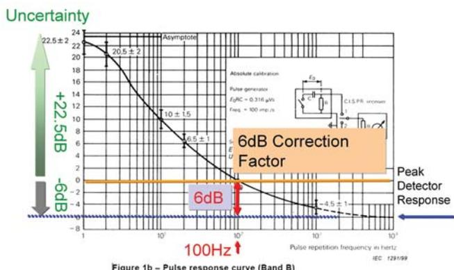
Figure 1 – Quasi-Peak Detector Correction
