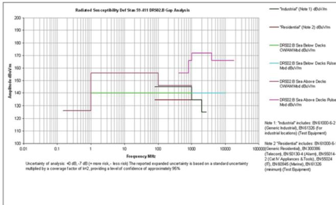
**Figure 10 – Example Radiated Susceptibility Gap Analysis – DRS02 – Sea Systems**
