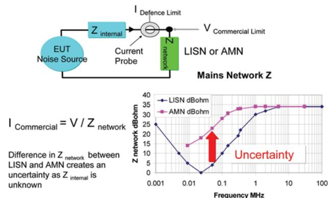
Figure 3 – Mains Network Correction
