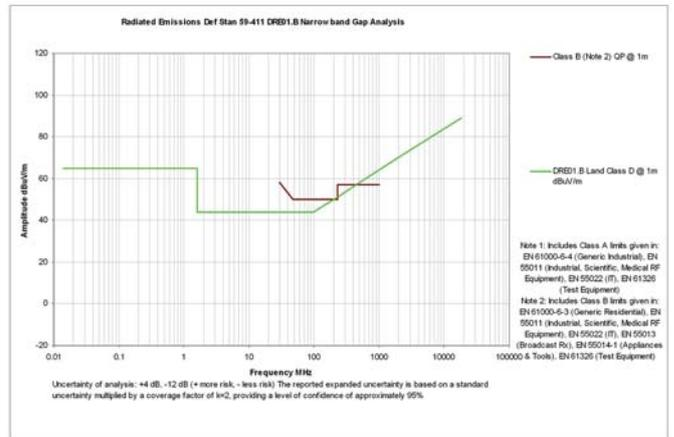
**Figure 7 – Example Narrowband Radiated Emission Gap Analysis – DRE01 – Land Class D vs Class B**
