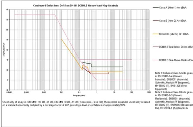
**Figure 5 – Example Narrowband Emission Gap Analysis – DCE01 Power – Sea Systems**
