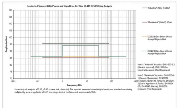
Figure 9 – Example Conducted Susceptibility Gap Analysis – DCS02 – Sea Systems
