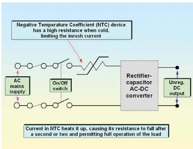
**Figure 6AY Reducing inrush current with an NTC**
