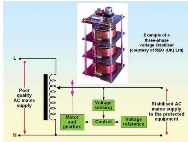
**Figure 6BR Servo-motor controlled ‘voltage stabiliser’ principles**
