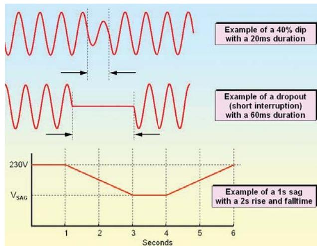
**Figure 6BE Examples of types of undervoltage events**
