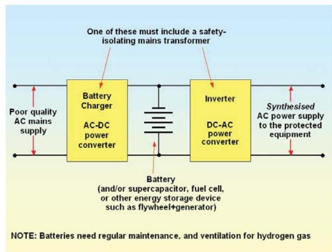
**Figure 6BS Principles of continuous-on-line double-conversion UPS**
