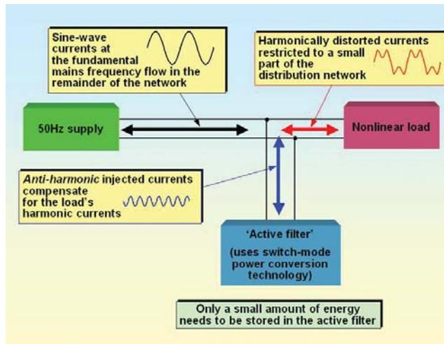
Figure 6BQ 'Active' mains filters – operating principles
