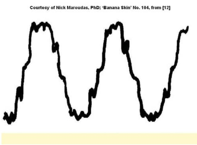
**Figure 6BM** An example of a mains waveform in a house in Israel in 2000
