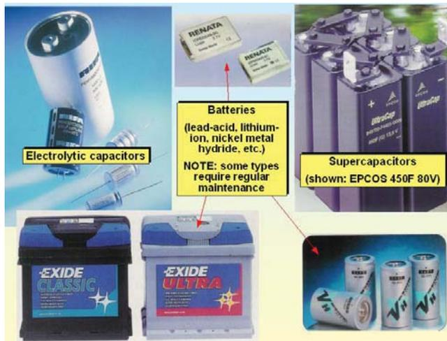
Figure 6BH Some examples of energy storage devices
