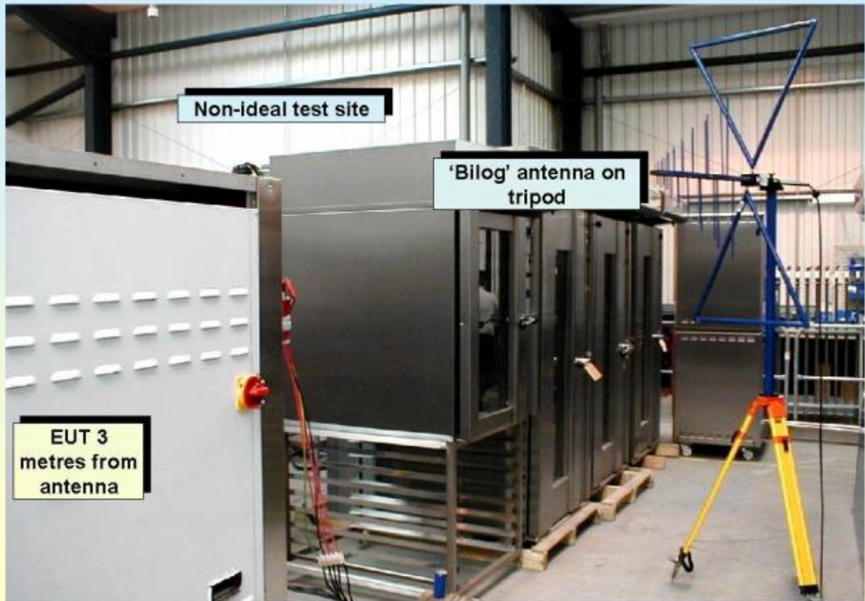
Figure 14 An example of on-site testing for radiated emissions
