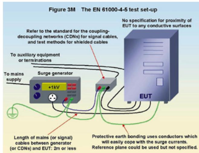
Anyone wishing to perform a surge test should have a copy of the relevant version of the basic test standard EN 61000-4-5, and follow it as closely as they need to for the test accuracy they require.
