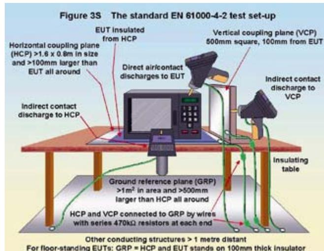
Anyone wishing to perform this type of personnel ESD test should have a copy of the relevant version of the basic test standard EN 61000-4-2, and follow it as closely as they need to for the test accuracy they require. Compliant ESD guns are easy to hire and relatively straightforward to use, and an example of one is shown in Figure 3T.
