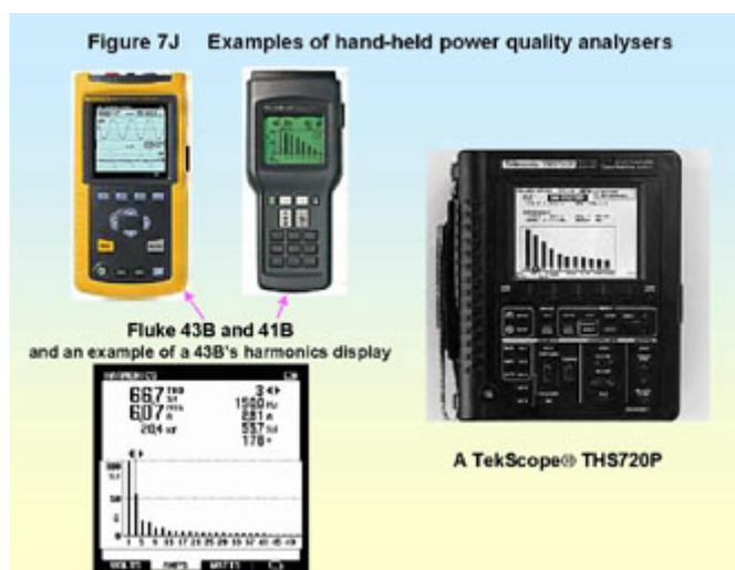
Unfortunately, the accuracy or display resolution or S/N available in some of these hand-held products might not be enough to check the compliance of a product's higher-order harmonics. Although these instruments say they will measure to the 31<sup>st</sup> or 50<sup>th</sup> or whatever, the EN 61000-3-2 limits for the high order harmonics just might not be discernible on their screens.
