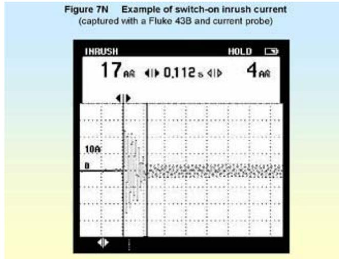
The mains source used may be a problem for inrush current tests. Current capability is very important when measuring inrush currents, and many types of 'clean' source might be current limited and unable to supply the current that the EUT would take from a real mains supply with the standard impedance. So when purchasing or designing a mains source it is best to ensure that it will source a short-term current which is very much larger than the EN 61000-3-3 limit for inrush current.
