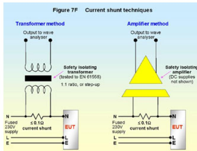
Step-up transformers must be used with fairly high-impedance loads so that they don't affect the accuracy of the  $0.1\Omega$  current shunt resistance. For example, with a 1:10 step-up and a 1% tolerance shunt the load on the analyser side should be  $10k\Omega$  or more.
