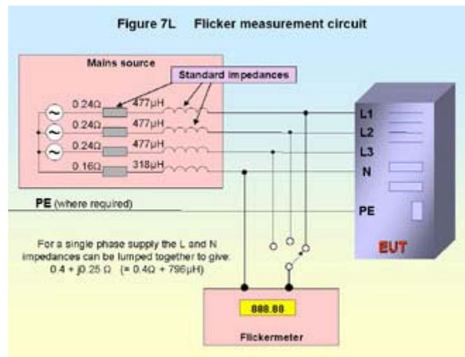
The accuracy of this set-up is required to be such that the relative voltage change can be measured with a total accuracy of better than  $\pm 8\%$  of the maximum allowed value. The measurement errors can be distributed between the reference impedance and the analyser as long as the total remains within this limit.
