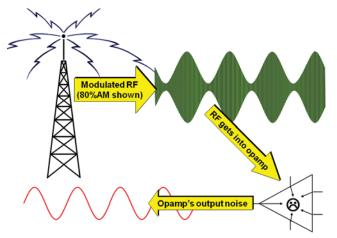
Figure 39 Example of RF demodulation of a radio broadcast
