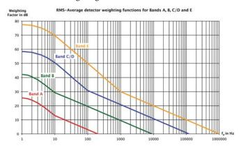
Fig. 2: RMS-Average weighting function for Band A, B, C/D and E
