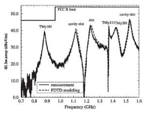
Figure 2 Comparison of the measured performance and EM simulation for a simple slot in a screened box
