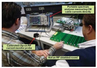
Figure 34 Quickly checking CM noise emissions without an EMC test chamber or site
