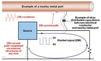
Figure 32 Example of stray capacitance coupling causing CM currents
