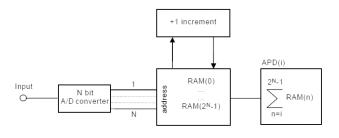
Fig. 4: Block diagram of APD measurement equipment
