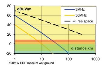
Figure 1 The signal strength of a 100mW source compared with the noise background. The red background corresponds to a "business" environment, the orange to "residential", the green to "Rural" and the blue to "quiet rural" at 10MHz
