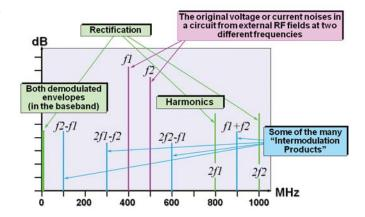
Figure 41 Example of the intermodulation of two frequencies in a semiconductor
