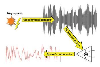
Figure 40 Example of RF demodulation of random RF noise
