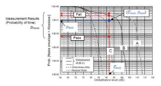
Fig. 5: APD weighting function for measuring the probability of occurrence over time (method 2)
