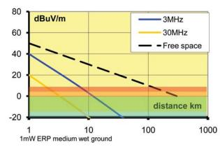
Figure 5 Field strength resulting from a 1mW transmitter. As in Fig 1 the red background corresponds to a "business" environment, the orange to "residential", the green to "Rural" and the blue to "quiet rural"
