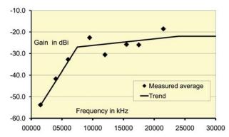
Figure 4 Average sky wave antenna "gain" for indoor sockets.
