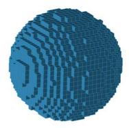
Figure 1. How the computer sees a dielectric sphere
