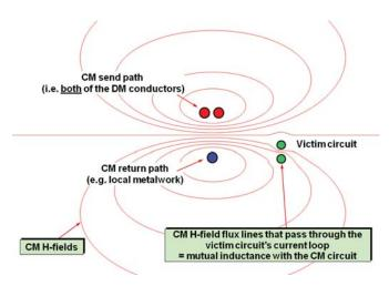
Figure 31 Example of H-field CM coupling
