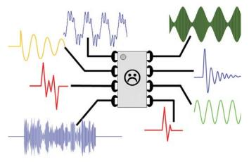
Figure 38 All IC pins are susceptible to RF demodulation
