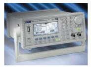
The TG5011 incorporates a pulse generator mode which provides a wide range of pulse width and delay independent of period. Pulse period can be set between 2000 seconds and 80 ns (0.5 mHz to 12.5 MHz) and the duty cycle can be as low as one in two billion. Rise and fall times (edge speeds) are also independently variable over a wide range.
