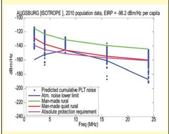
Figure 6 Predicted cumulative PLT noise parameters for example with receiver in Augsburg, compared to established background noise levels.
