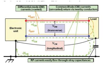
Figure 30 The loops enclosed by DM wanted signals/power and by unwanted CM
