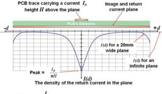
$I(d) = \frac{I_0}{\pi H \{1 + (D/H)^2\}}$  for a long straight trace over an infinite plane
