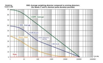
Fig. 3: RMS-Average compared to Average, Quasi-peak and Peak detector
