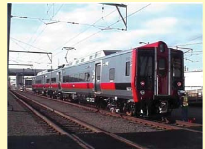
One of the Metro-North Railroad’s eight new M-8 railcars.
